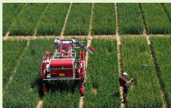
Two types of phenotyping devices : the large phenomobile, and the 'literal' (a light and easy-to-carry system). Credit : Arvalis and Hiphen
