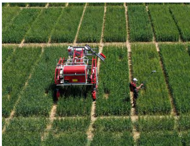
Figure 14 Two types of phenotyping devices : the large phenomobile, and the 'literal' (a light and easy-to-carry system). Credit : Arvalis and Hiphen.
